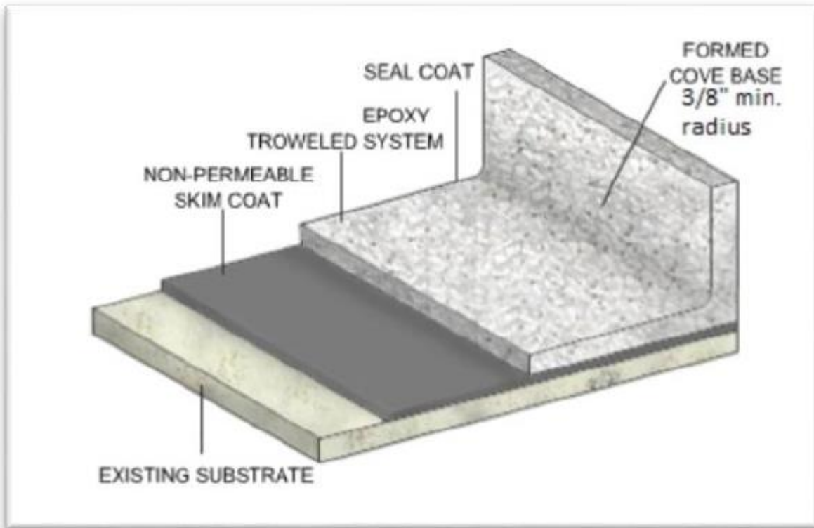
Fig. 3 Troweled on Epoxy Floor and Cove Base Installation (Troweled on epoxy floor specifications must indicate that the material is USDA/FDA approved for use in a food facility and is acid and grease resistant)
